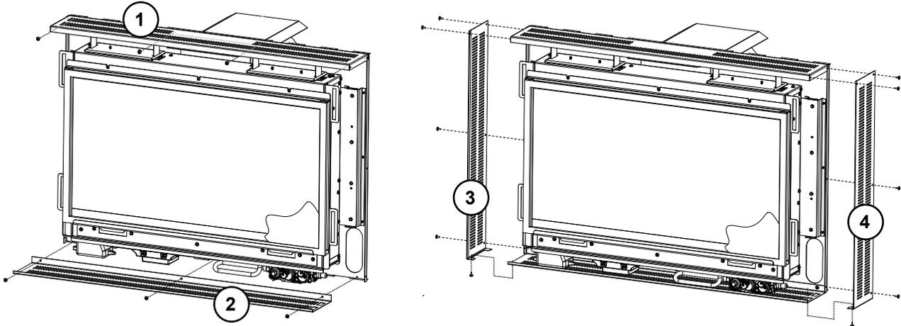
Secure the housing panels as illustrated using the 17 #8 X 3/8" screws supplied.
