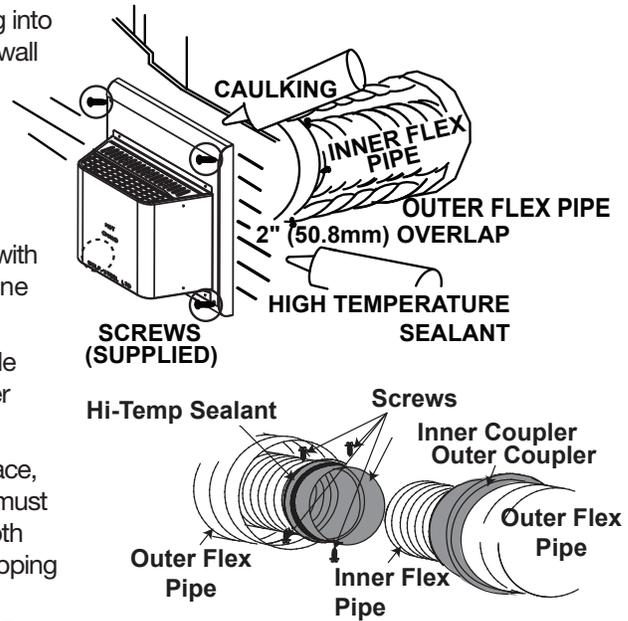
**The air terminal mounting plate may be recessed into the exterior wall or siding no greater than the depth of its return flange.**
