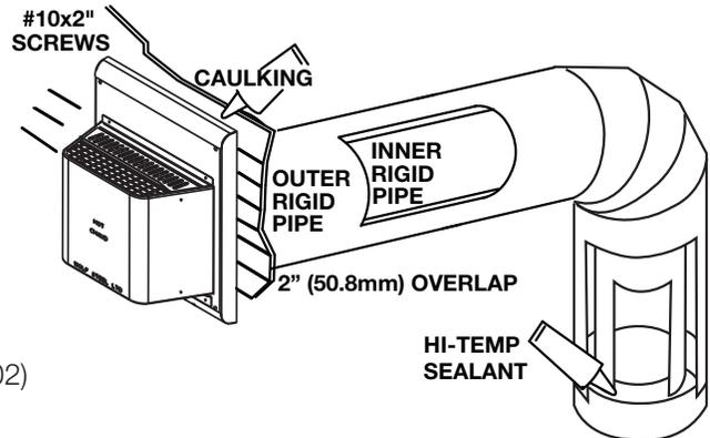
**The air terminal mounting plate may be recessed into the exterior wall or siding no greater than the depth of the return flange.**
