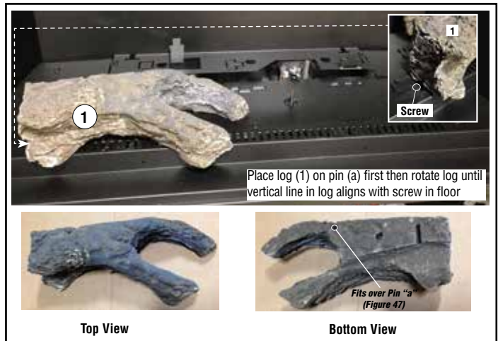
Figure 48 - Place front left log (1)
