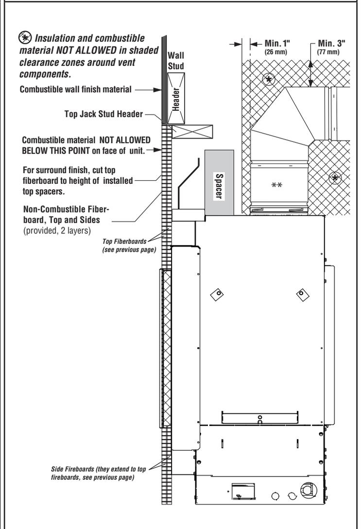
\*\* 6" straight vent section required before 90° elbow
