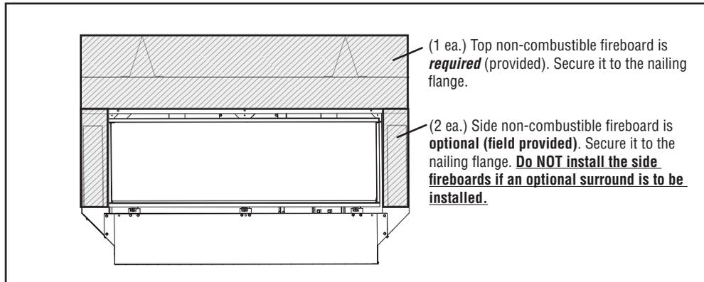
**NOTE:** The non-combustible fiberboard may be skim coated as a finish material, however, other types of non-combustible board may provide a more durable surface.
