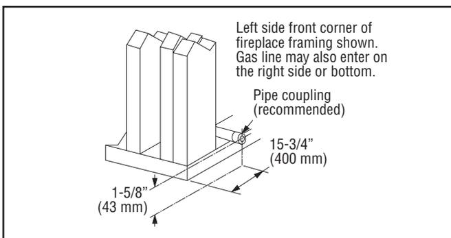
**Figure 10 - Routing the gas line into the fireplace**
