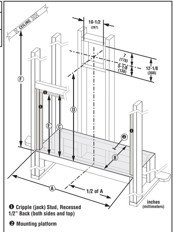
**Table 11 - Fireplace Framing Specifications—Corner Installation with Horizontal Termination**
