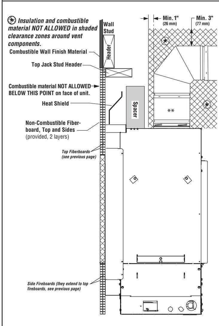
**Figure 39 - Noncombustible Material with Surround—Profile View**
