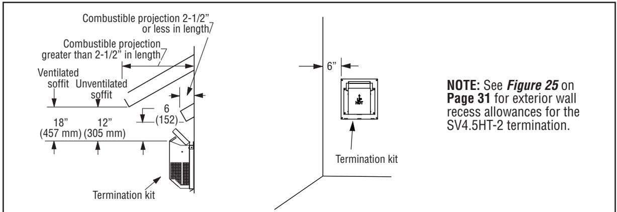
**NOTE:** See **Figure 25** on **Page 31** for exterior wall recess allowances for the SV4.5HT-2 termination.
