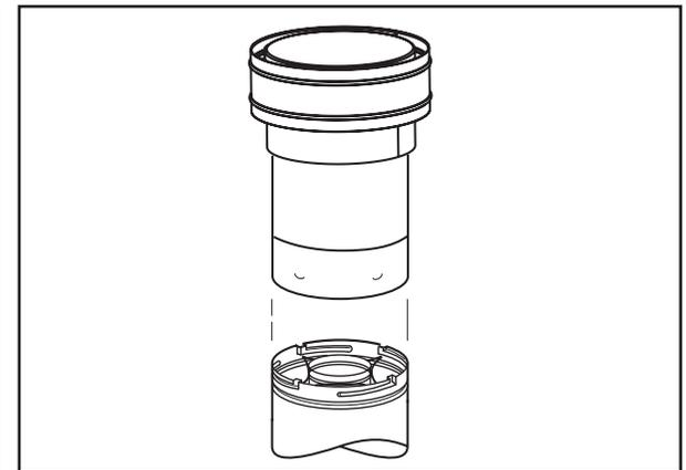
12. **Install the vertical termination**—Extend the vent sections to the correct height (**Table 6**). The SV4.5CGV-1 Vertical Termination (**Figure 21**) installs in the exact same fashion as any other Secure Vent® section.
