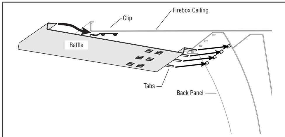
2. While sliding the tabs into the slots, slide the front lip of the baffle under the clips in the firebox ceiling.
