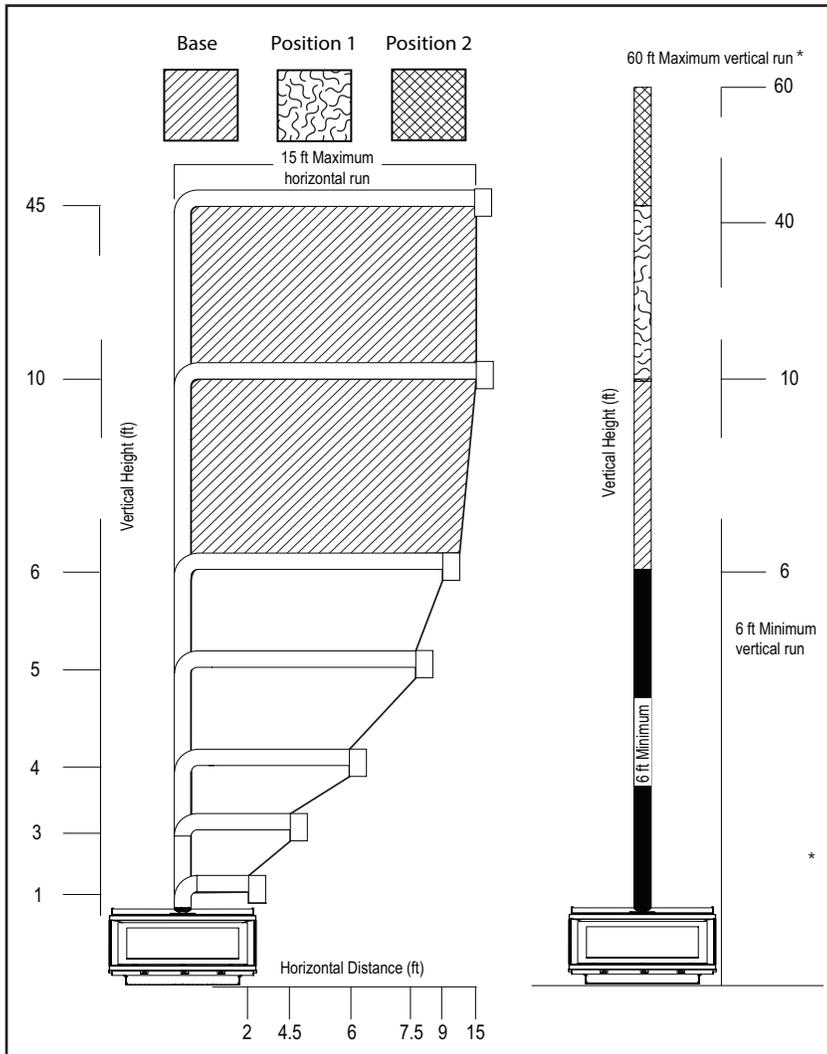
**Figure 12 - Vent restrictor installation, Top vent**
