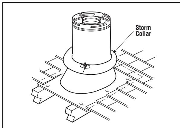
**Figure 21 - Installing the Vertical Termination**
