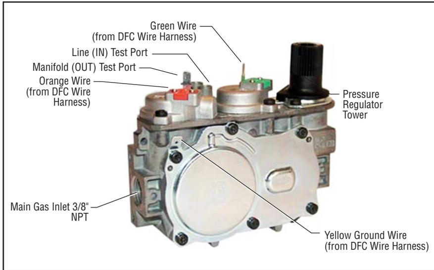
The SIT gas valve in this fireplace has a 3/8" NPT thread main gas inlet and outlet. Test gauge connections are provided on the front of the electronic gas control valve (identified IN for the inlet and OUT for the manifold side).
