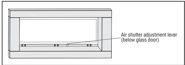
1. Move the adjustment lever (**Figure 34**) down to decrease air flow and up to increase it. Position the air shutter to the factory setting (**Table 26**).
