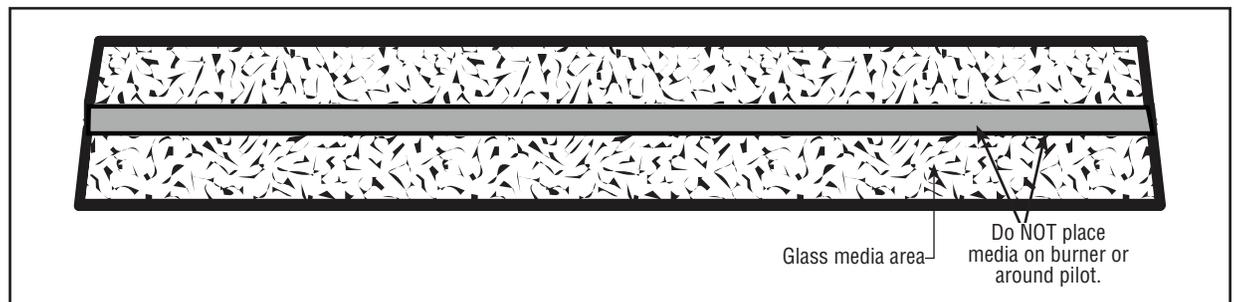
**NOTE:** It is important to ensure proper media placement per the manual when installing these units. Verify pilot flame is not obstructed. Ensure media does not fall through the pilot hole in the floor. See *Verifying Appliance Operation* on **Page 38**.
