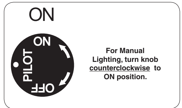
Fig. 37-3 Control knob detail (ON)
