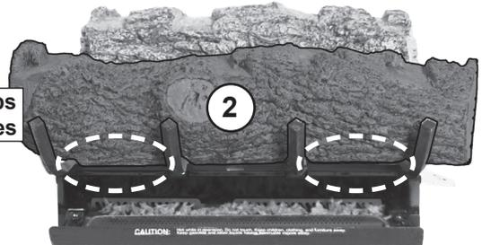
Place the front log (log #2) as shown. The underside of the log has two tabs that insert into the holes found on the burner. The cutouts found on the underside of the log will align over the grate fingers. ENSURE THE LOG RESTS FLAT ON THE BURNER/GRATE.
