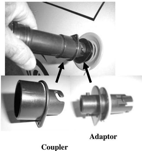
If you will be using another inflation device with a larger nozzle, use the 1 ¼" diameter coupler (included) between the valve adaptor and the hose of your inflator. Make sure the hose is attached to the blower port of the vacuum for inflation. Insert the adapter into the air valve and lock into place by turning clockwise.
