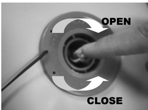
To lock open valve, depress the stem and rotate  $\frac{1}{4}$  turn clockwise. To close valve, depress the stem and rotate  $\frac{1}{4}$  turn counter-clockwise. The valve stem should be in the depressed position while inflating. Replace the cap on valve after inflation to ensure air tight seal.
