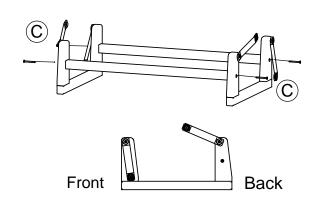
Note: The direction of the pillars on the base. The angled edges should be facing the back when assembled
