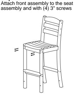
Step 2 Attach back leg assembly to seat assembly using (4) 3" screws
