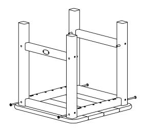
Step 2: Now loosely attach braces using the remaing (4) 2-1/4 screws Afterwards, turn table upright and tighten all screws.
