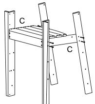
Step 3 Attach back to seat using (2) .27x2" screws
