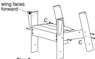
Step 3 Attach back to seat using (2) .27x2" screws
