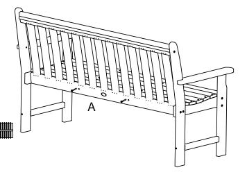
Step 4 Attach angle brace to front leg then seat using (4) 8x2" screws
