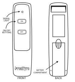
The transmitter operates on a 12V battery (included) made specifically for remote controls and electronic lighters. Install the 12V battery supplied with the unit into the battery compartment.
