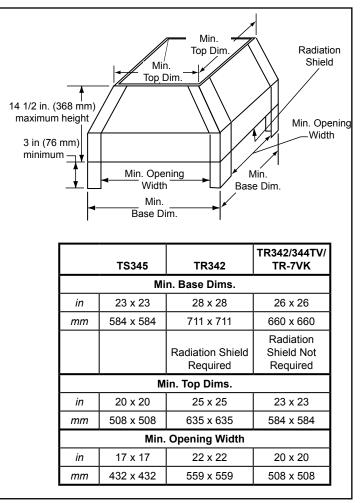
TR342/344 caps require radiation shield unless installed partially above the shroud. The TR cap must be raised to the minimum dimensions (or greater) above the shroud. Refer to Figure 6.3.
