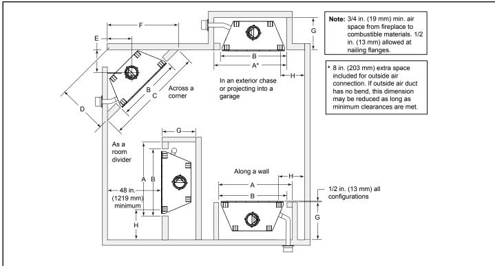
Note: Measurements are FRAMING dimensions only and do not include drywall either in the cavity or on the interior walls.
