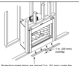
Protective metal strips are placed 2 in. (51 mm) under the front of the fireplace and must extend beyond the front and sides of fireplace opening by 2 in. (51 mm).
