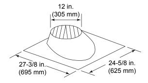
RF370 Roof Flashing
