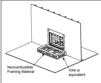
Figure 7.6 Raised Platform Hearth Extension-Framing
