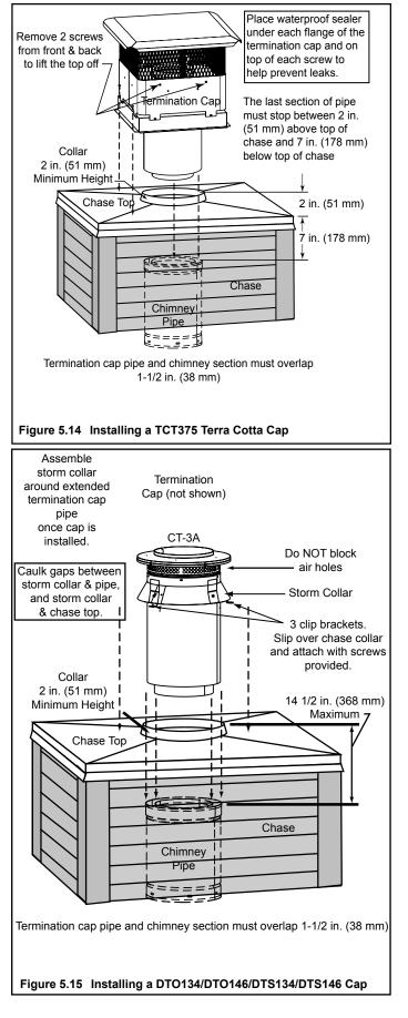
**WARNING! Risk of Fire!** Shrouds must be constructed as specified. Improper construction may overheat chase top.
