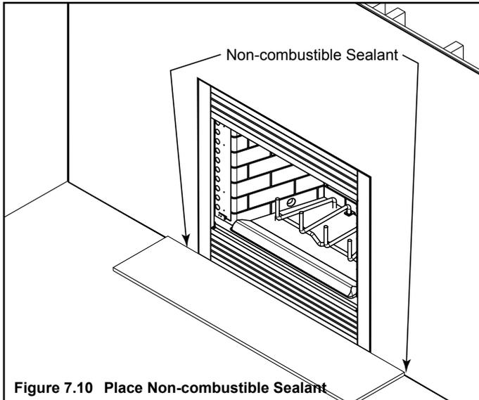
Figure 7.10 Place Non-combustible Sealant
