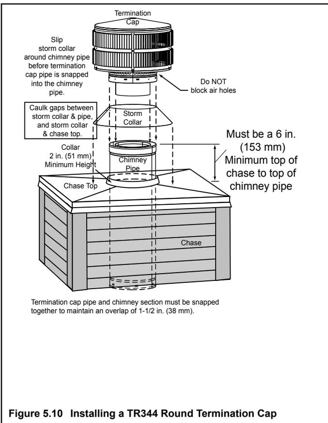
Figure 5.10 Installing a TR344 Round Termination Cap
