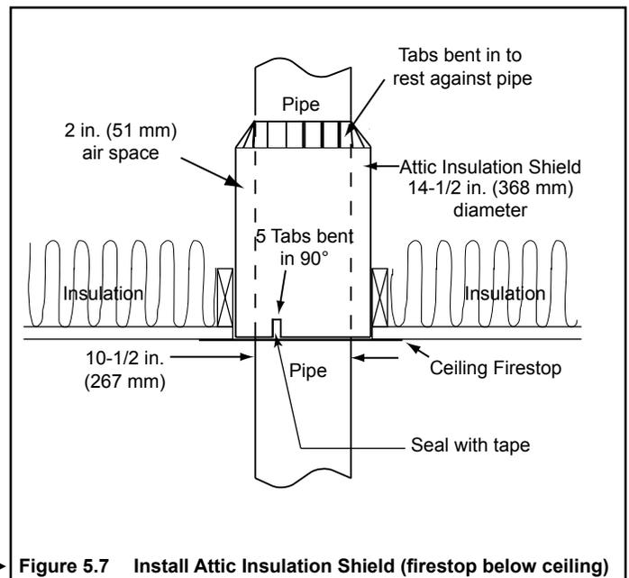
► **Figure 5.7 Install Attic Insulation Shield (firestop below ceiling)**
