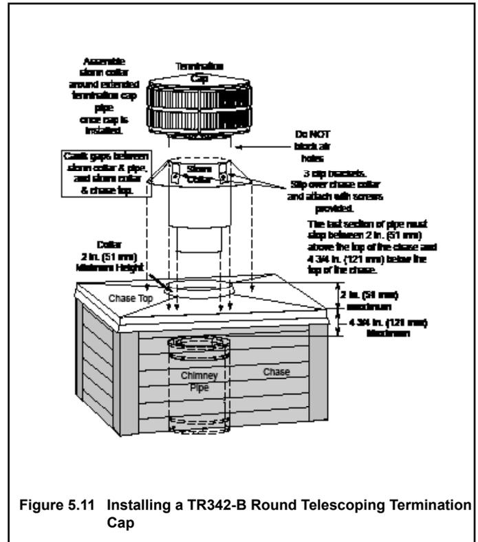
Figure 5.11 Installing a TR342-B Round Telescoping Termination Cap
