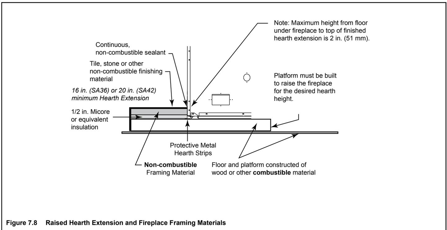
Figure 7.8 Raised Hearth Extension and Fireplace Framing Materials
