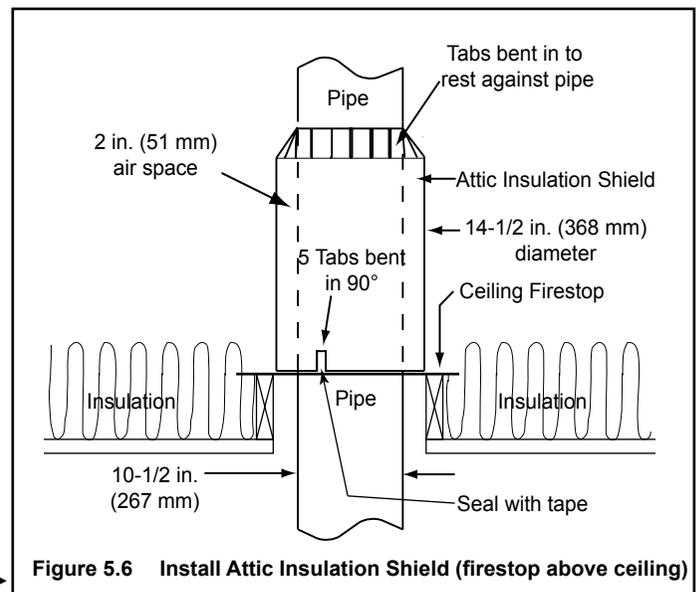
► **Figure 5.6 Install Attic Insulation Shield (firestop above ceiling)**
