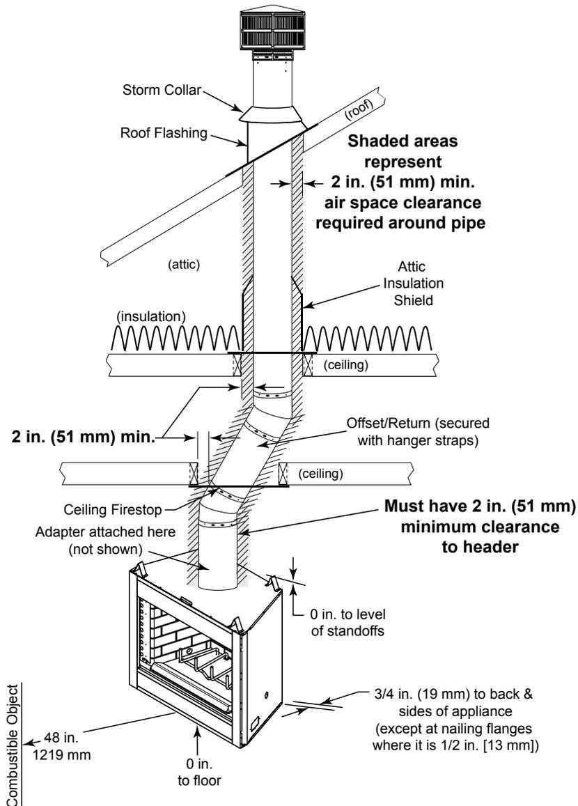
Figure 3.2 Clearances to Combustible Materials
