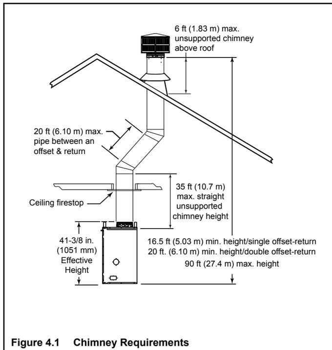
**Figure 4.1 Chimney Requirements**
