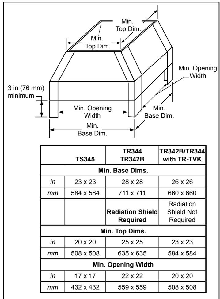
TR342 caps require radiation shield unless installed partially above the shroud. The TR cap must be raised to the minimum dimensions (or greater) above the shroud. Refer to Figure 6.3.
