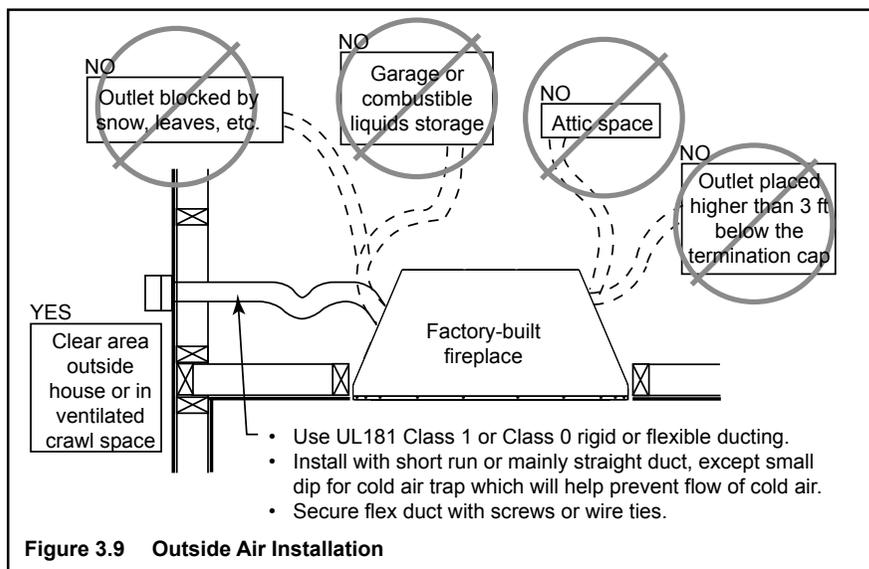
Figure 3.9 Outside Air Installation
