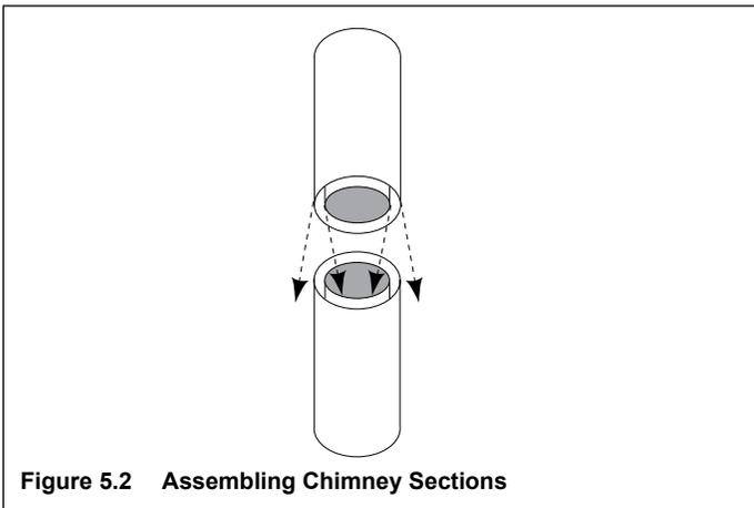
Figure 5.2 Assembling Chimney Sections
