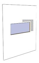
3. Secure fire unit to the finished framed opening with the provided large washer head screws. Make certain that at least 4 of the screws are driven in to a solid backing. Fireplace will stand proud of the finished wall opening by 1 1/8 inches, this area must not be blocked by any additional trim, tile, etc. as this will block proper air flow. This is a semi-permanent installation. Remove screws to relocate.
