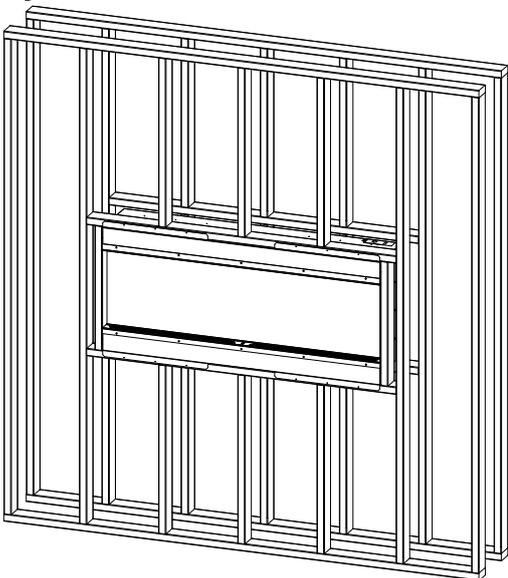
5. **Mask the exposed fire unit during the drywall process.** Install drywall to the drywall stops on the perimeter of the fire box. For more information on the drywall stops see the Product Guide on page 4. Decorate as desired.
