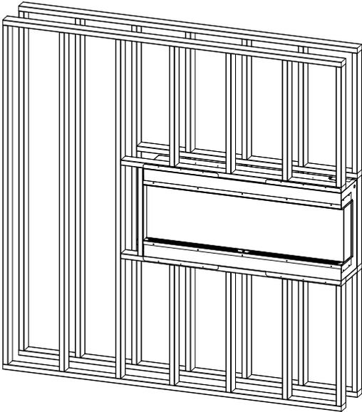
4. Install the fire unit in the framed opening with a minimum 1 ¼ drywall screws to secure the unit.
