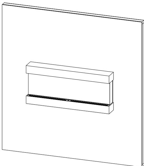
4. **Firebox must be covered with material of choice. Mask the exposed fire unit during this process.** Install drywall, tile or material of your choice to the drywall stops on the perimeter of the fire box. For more information on the drywall stops see the Product Guide on page 4. Decorate as desired.
