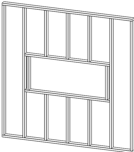
1. This installation is optimized for a 2x4 framed wall. Prepare the framed opening according to the height and width of the chart on page 7. Provide a dedicated flexible 15 amp 120 volt circuit for hard wire installation.
