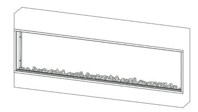
3. Place the logs on top of the acrylic crystals.
