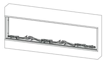
4. The front glass can now be installed, by installing bottom of glass in track, then tilt towards fireplace.
