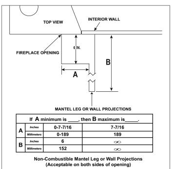
If using heat management please refer to the fireplace installation manual for framing guidelines and reduced mantel clearances. Additional information on venting, TV clearances, finishing requirements, fronts, etc can be found in the installation and owner's manual
