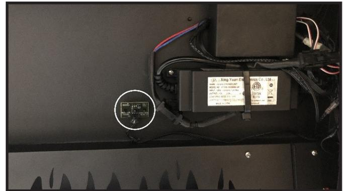
Figure 11 Receiver Board Removal
