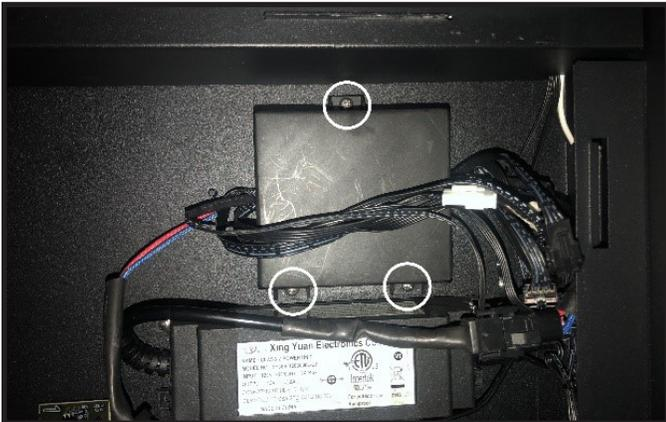
Figure 12 Control Board Removal
