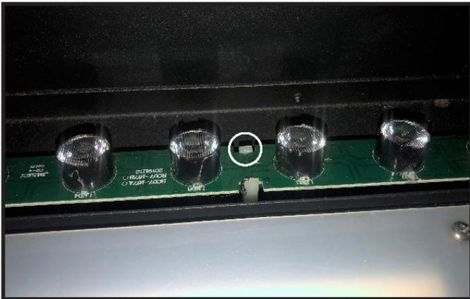
Figure 19 LED Board Removal
