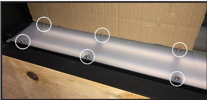
Figure 7 Fuel Bed cover Removal
