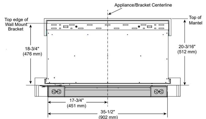
An electrical receptacle may be discretely located under the bottom mantel. When planning the location of the appliance, special care is required to ensure the wall mount bracket is located a sufficient distance above the electrical receptacle.
