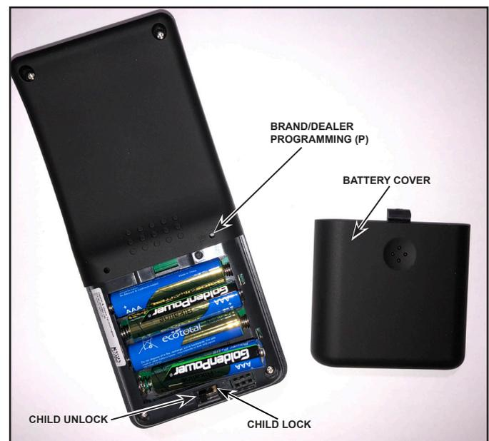
Figure 12 Install Batteries & Child Safety
