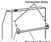
Stand-Out Tab Mounting Bracket (attached to wall)
