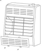
Figure 7 - Removing Lower Front Panel of Heater
