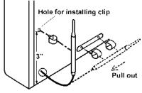
Figure 5 - Moving Thermostat Sensing Bulb
