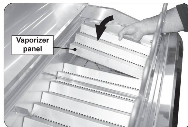
Fig. 25-2 Install vaporizer panels
