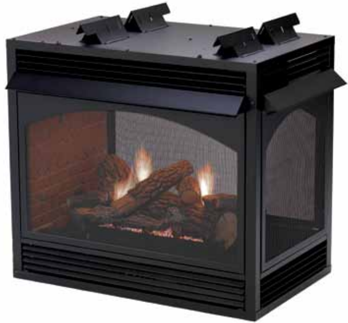
The Vail Premium 36-inch Peninsula Vent-Free Fireplace includes a 38,000 Btu Slope Glaze Vista Burner, plus fixed screens, louvers, and hoods on three sides. Requires Rock Creek refractory log set. Also available in See-Through model with two open sides
