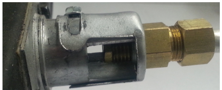
Air Shutter - C NOTICE: Orifice shield removed for photo clarity.
