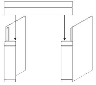
3. Use (4) 1-1/4" drywall screws per side to attach gussets to the side assemblies and breastboard assembly.
