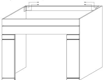
6. Attach unit to studs in the wall through the rear brace using (2) 2-1/2" drywall screws provided.
