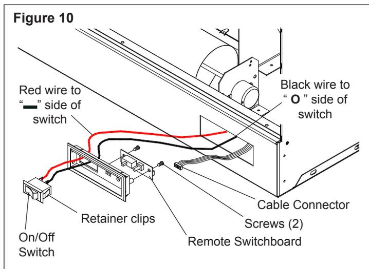
12. Remove the On/Off Switch by squeezing the two (2) retaining clips on either side of the switch, from within the firebox, then push out the front of the unit.
