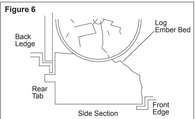
9. Install the Log Set Assembly by placing the front, bottom edge of the Ember Bed in the track behind the control panel. Once in place, push down on the back edge of the Ember Bed until the rear tab snaps into place under the Partially Reflective Glass (Figure 6).
