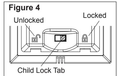
3. Move Child Lock tab back to the left to unlock the remote control.
