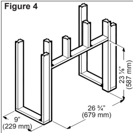
Dimplex mantel, the fireplace must be installed in an enclosure with the following **minimum** internal/opening dimensions (Figure 4).
